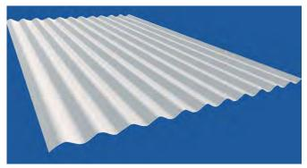
Normal Corrugation 110 (NC 110) is a sinusoidal profile with 11 corrugations and a pitch (distance between any two crests) of (76 +/- 2 mm) hence its name, and is the oldest commonest of all profiles, mainly used for roofing and walling especially in domestic applications.
